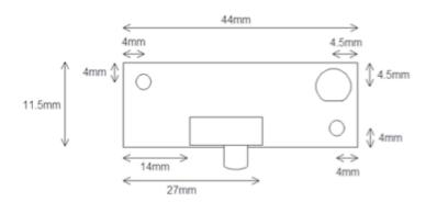
The 2 mounting holes are 3.3mm diameter.
