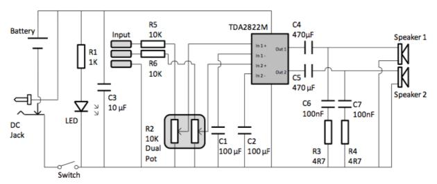
At the centre of the circuit is an audio amplifier Integrated Circuit or IC. Inside the IC are lots of transistors, which are connected together to allow the small input signal to be amplified into a more powerful output that can drive a speaker.
