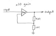
With an infinite gain the amplifier is no good to amplify audio, which is where the feedback comes in. By making one of the input a percentage of the output the gain can be fixed, which allows the output to be a copy of the input but bigger. Now when the two inputs are compared and the output is adjusted, instead of it going up or down until it reaches 0 volts or V+, it stops at the point when the two inputs match and the output is at the required voltage.
