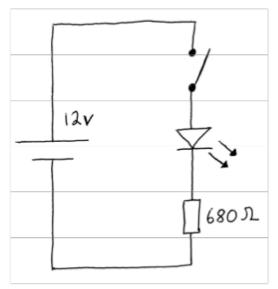
The circuit diagram for the torch is shown on the left. It is a very simple circuit, powered by a 12 volt battery.
