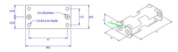
All dimensions in mm x4 holes 3.3 mm diameter x2 LEDs 5mm diameter
