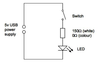
The circuit diagram for the USB lamp is shown on the left. It is a very simple circuit. The 5V that powers the circuit is supplied from the USB connector.
