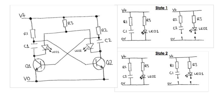
The circuit has two states which it alternates between. In each of the states one of the LEDs is on while the other is off.
