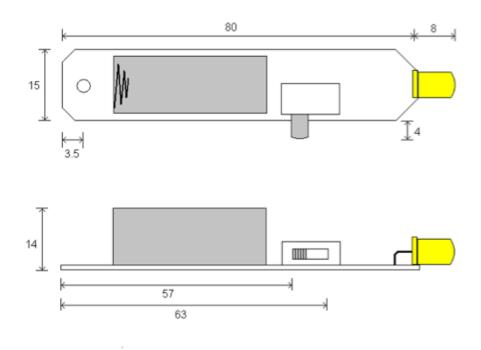
All dimensions in mm. x1 mounting hole 3.3 mm diameter. The diameter of the LED is 5 mm.
